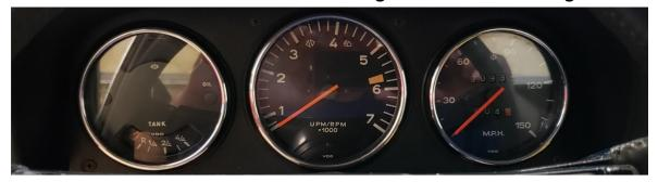
These trim rings can be installed without removing the gauges. No glue or tape is needed Instruction:
