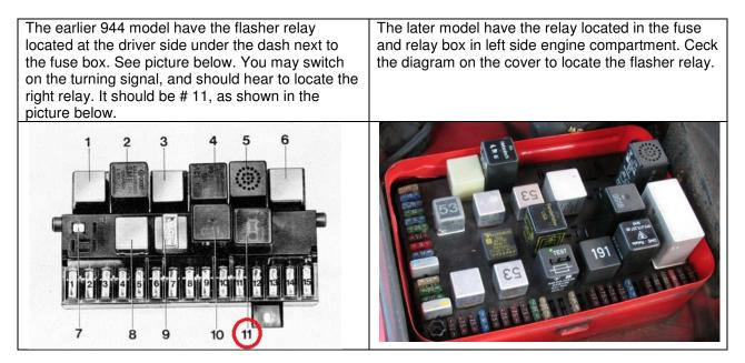
Remove the relay and replace it with the new one. ATTENTION: Do not use the new relay with the standard bulbs, it can damage the new flasher relay.
