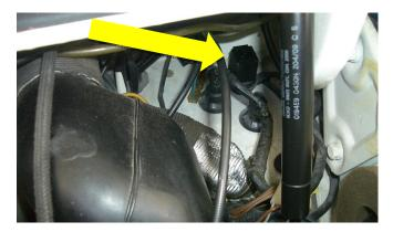
Remove the relay and replace it with the new one. ATTENTION: Do not use the new relay with the standard bulbs, it can damage the new flasher relay.
