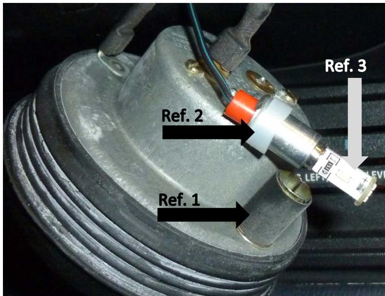
The clock and the Gas/Oil gauge have only one bulb, and the depth for the light bulb on the clock is less as on the other gauges.
