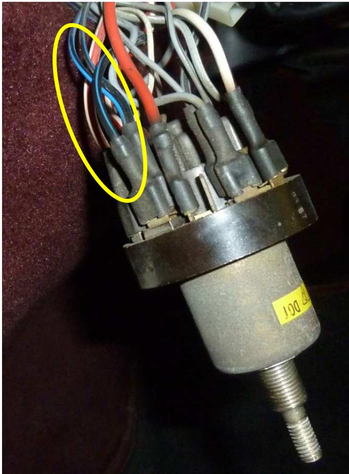
The fuse will be connected between the switch and the black-blue wire, connector No. 58a.
